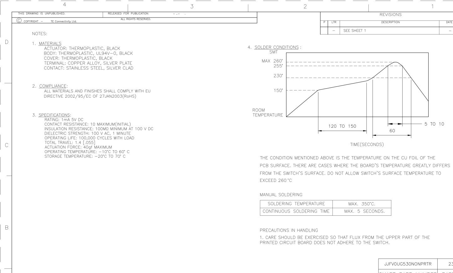
SMART PART NUMBER PART NUMBER 07MAR2018 THIS DRAWING IS A CONTROLLED DOCUMENT. <del>S</del>TE TE Connectivity Ltd. 07MAR2018 ALEXANDER SHARPE TOLERANCES UNLESS OTHERWISE SPECIFIED: DIMENSIONS: ALEXANDER SHARPE mm [INCHES] SWITCH, DETECTOR, JJF SERIES, 4.7X3.8mm, PRODUCT SPEC VERTICAL, SMT ± 0.20 [.008] APPLICATION SPEC PLC CAGE CODE DRAWING NO PLC RESTRICTED TO PRELIMINARY WEIGHT 00779 **C**-2331367 SHEET CUSTOMER DRAWING 2 OF 3
