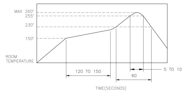
THE CONDITION MENTIONED ABOVE IS THE TEMPERATURE ON THE CU FOIL OF THE PCB SURFACE. THERE ARE CASES WHERE THE BOARD'S TEMPERATURE GREATLY DIFFERS FROM THE SWITCH'S SURFACE. DO NOT ALLOW SWITCH'S SURFACE TEMPERATURE TO EXCEED 260°C
