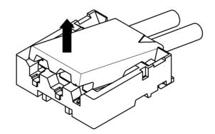
③Lift up to the upper direction and positive lock is released. Removal completes.
