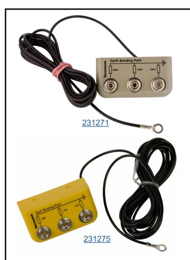
"The protection of ESDS [ESD sensitive item] is accomplished by providing a ground path to bring ESD protective materials and personnel to the same electrical potential. All conductor and dissipative items in the environment, including personnel, shall be bonded or electrically connected to a known ground or common connection point [Earth Bonding Point]." [CLC/TR 61340-5-2 User guide clause 4.4.1 Grounding/bonding systems Introduction]
