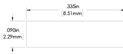
RECOMMENDED SOLDER PAD SIZE (.090 [2.29] X .335 [8.51])
