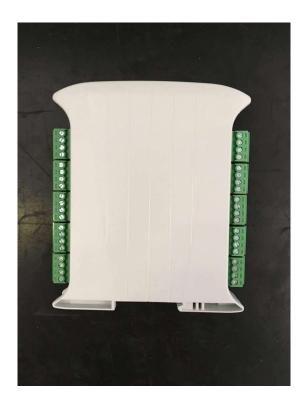
Digital Optoisolated input module. Converter (12Vdc/Vdc to 220Vac) to 5-24Vdc
