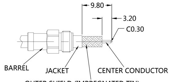
OUTER SHIELD (IMPREGNATED TIN) RECOMMENDED STRIPPING DIMENSIONS
