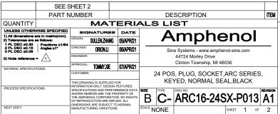
24 POS, PLUG, SOCKET, ARC SERIES, KEYED, NORMAL SEAL, BLACK
