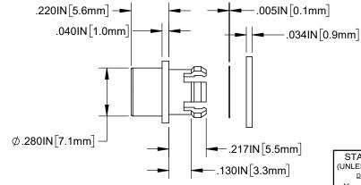
RECOMMENDED LENS MOUNTING HOLE PANEL THICKNESS: .118IN [3mm] MAX. **CUSTOMER USE DRAWING** STANDARD TOLERANCE
