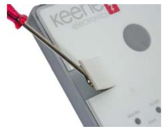
Replacement front panels are available, (part number KLAB20DSFP)
