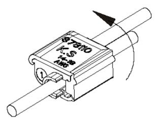
Insert unstripped tap wire completely into tap port.
