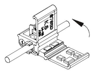
Insert unstripped tap wire completely into tap port.
