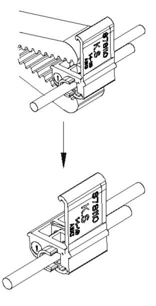
Make connection with pliers held perpendicular to wires by driving "u" contact down flush with top of connector.
