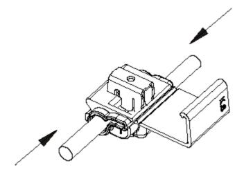
Make connection with pliers held perpendicular to wires by driving "u" contact down flush with top of connector.
