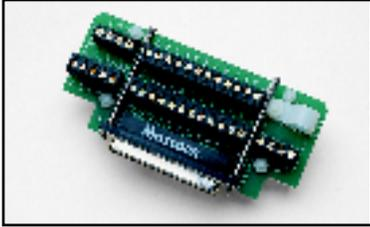
**STC-37:** Direct Screw Terminal Connector (37 pin). The STC-37 plugs directly onto the I/O connector at the back of the PC. All lines are brought out to screw terminals.
