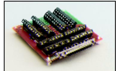
**STP-3140:** Screw Terminal Panel. Brings all KPCI-3140 signals out to external screw terminals. The STP-3140 comes with nylon standoffs, making it ideal for placing on a desktop or mounting in custom panels. Requires the CAB-307 and CAB-308 cables (1m/39").
