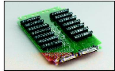
**STP-3110:** Screw Terminal Panel. Mounts on a panel and includes nylon standoffs for tabletop applications. For use with KPCI-3110 and -3116 data acquisition boards. CAB-307 and CAB-308 cables are required.
