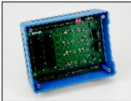
**STA-MB:** The STA-MB Screw Terminal Accessory provides sockets for 4 MB-Series modules. Two parallel 37-pin D male connectors provide interfaces for DAS boards and accessories. The MB-Series module inputs and outputs as well as the I/O connector pins are brought out to screw terminals. You then wire the MB-Series outputs to pins on the I/O connectors according to the requirements of your application.
