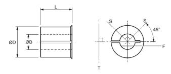
Bore For optimum fastening, install HUCO-LOK bore adaptors as shown.
