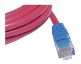
Wiring is cross-over T568A to T568B which is used to daisy-chain switches/hubs or for direct connection of 2 computer network interface cards. Red cord jacket with Blue injection-moulded boots minimises chance of confusion with straight-thru cords. 2 Metres in length.
