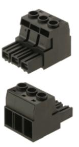
High-performance female connector with the tried-and-tested, guaranteed zero-maintenance, Weidmüller steel clamping yoke. Side-by-side mounting without losing any poles or with patented multifunction flange for secure, fast fixing without tools. Maximum connection and operating reliability thanks to pin arrangement that prevents wrong connections or wrong wiring, unique coding diversity, 4-point silver contact.
