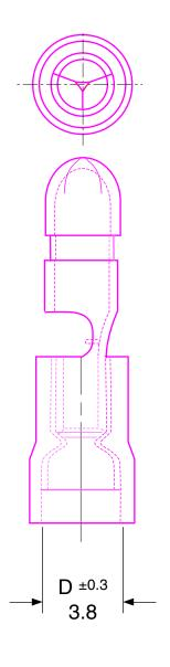
Max Electric Current: 22-16 AWG / 10 Amp Max Electric Rating: 75° C / 300 V max
