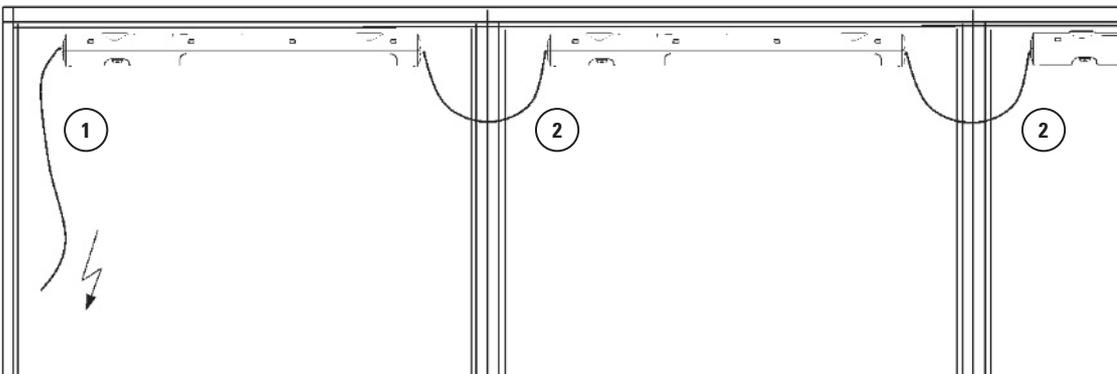
This illustration shows the LED 025 lamp in a daisy chain application. The lamps are conveniently connected via quick connection plugs – up to 10 lamps max. can be daisy-chained this way. The snap lock connectors ensure a stable electrical connection even if subjected to heavy vibration. The connection example shows a 230VAC application, using the following cables: connection cable with female connector, Art. No. 244356 (1); daisy chain extension cable with 2 connectors, Art. No. 244358 (2).
