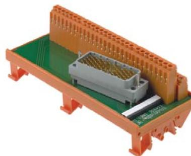
Weidmüller's passive interface units are used for adapting hermaphrodite ELCO multi-pole connectors, for input and output, to screw terminal systems. The hermaphrodite contact is a fork-type contact that is identical in design on both sides of the connection, but with one fork turned through 90° to engage with the other.
