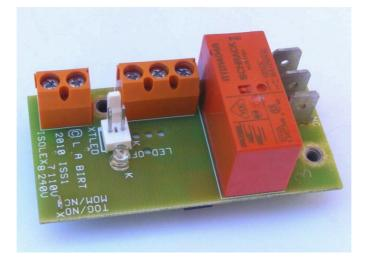
At last, a 21<sup>st</sup> century, low cost alternative **to air switch systems and tubing**. These AC powered, miniature (60 X 30 mm) units utilise advanced ferro-magnetic technology to provide **full galvanic isolation to connected electrical switches**. The novel, low impedance technique, passes near zero current through the connected switch creating a safe, earthed **'electric free'** circuit.
