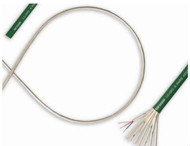
Van Damme Green Series Digi Grade cables have been specifically designed for the accurate transmission of AES/EBU digital audio signals. Low capacitance and stable characteristic impedance ensure that signals remain error and jitter free over long distances. This also makes this cable range suitable for other critical data transfer applications such as RS422, midi and timecode. Also suitable for balanced analogue audio use.
