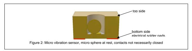
The unidirectional sensor version MVS1006.01 is open at rest, when mounted upside down position, so that the micro sphere is on the top side of the sensor, which has no contact.
