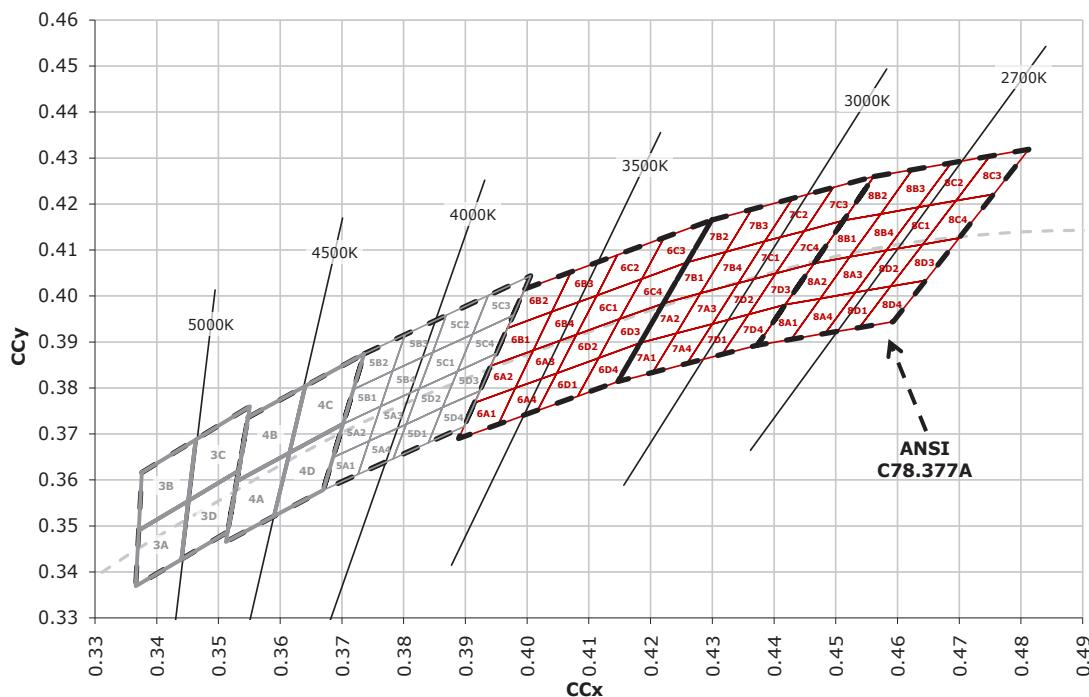
The following tables of order codes list flux minimums and chromaticity regions for XLamp XM-L LEDs. For other flux and chromaticity combinations, contact Cree or an authorized distributor.
