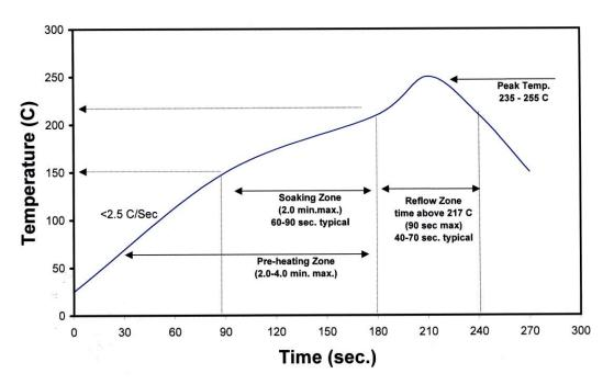
Figure 5: Reflow soldering profile for lead free soldering.
