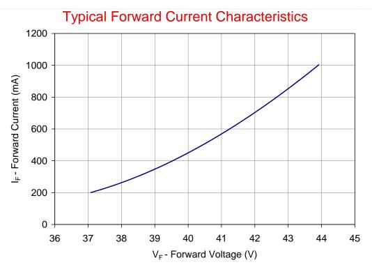
Figure 9: Typical forward current vs. forward voltage @ T<sub>c</sub> = at 25°C.
