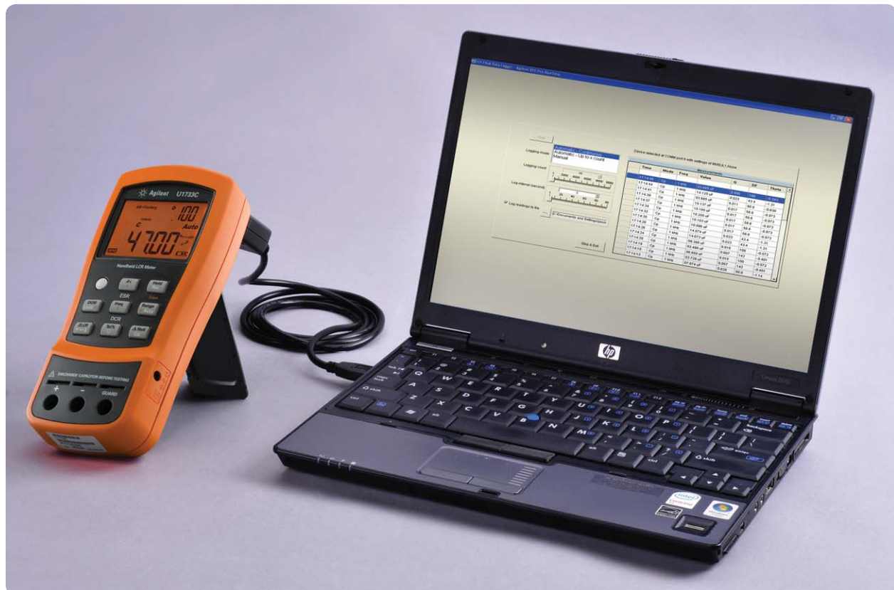
Figure 1. Automate the recording of continuous readings when you hook the U1731C/U1732C/U1733C to a PC
