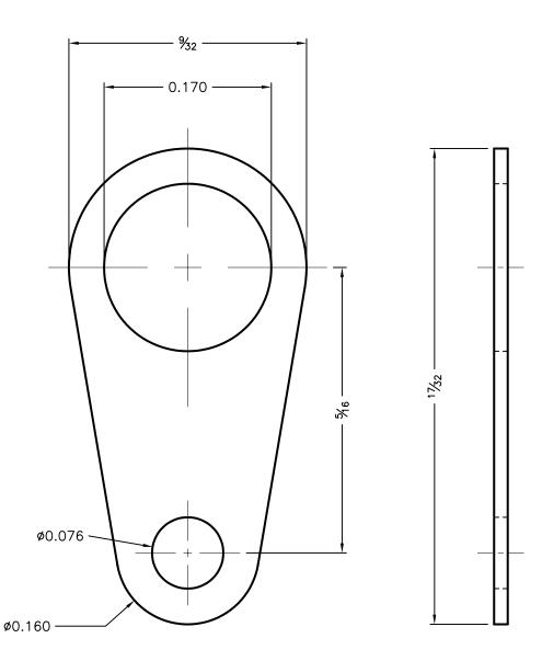
Material: 0.015 Thick Copper, Tin Plate
