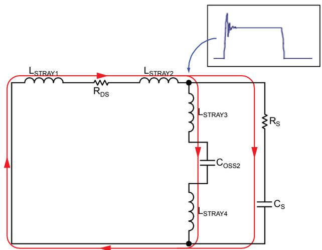
**Figure 6. Snubber Circuit**
