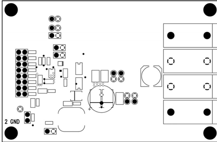
Figure 13. MIC2166 10A Evaluation Board Mid-Layer 1 (GND Plane)
