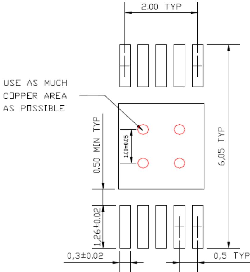
Red circle indicates Thermal Via. Size should be .300-.350 mm in diameter, 1.00 mm pitch, and it should be connected to GND plane for maximum thermal performance.
