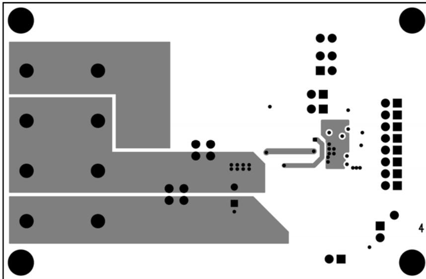
Figure 12. MIC2166 10A Evaluation Board Bottom Layer
