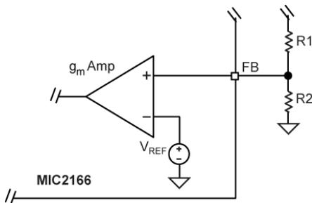
Figure 8. Voltage-Divider Configuration
