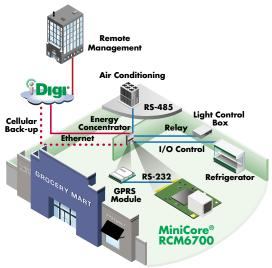
**Potential Applications:** Smart metering, energy management, building automation & security, point-of-sale, medical, motor control
