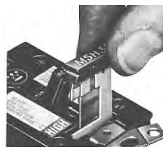
Heater Element Installation
