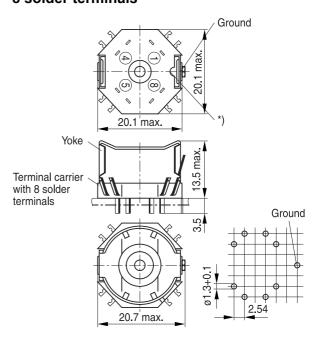
\*) This recess must be on the side of the grounding pin to ensure that the yoke locks in position.
