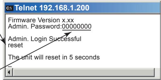
**Figure 3.3 Telnet Login into the iServer**
