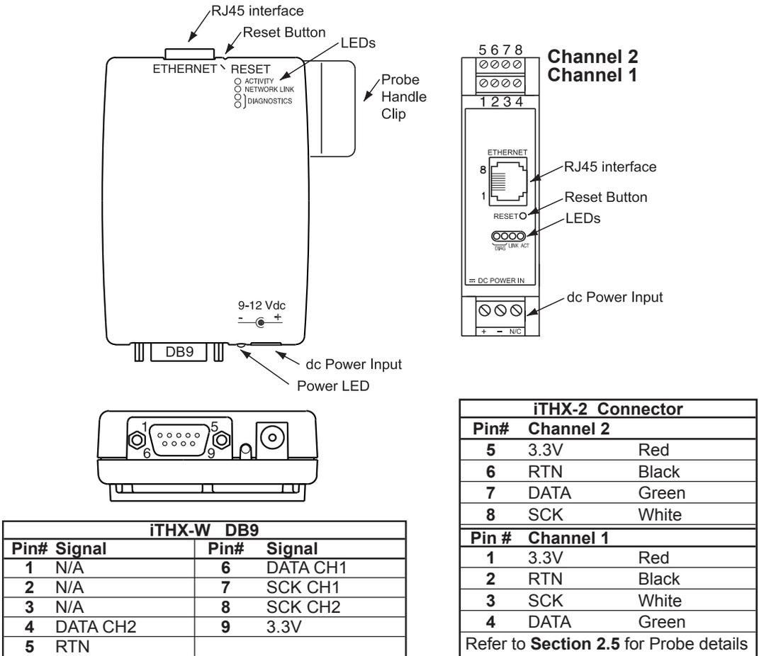
Figure 2.5 Parts of the iServer Unit
