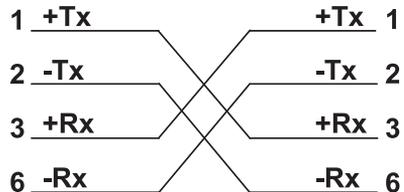
Figure 2.7 10Base-T Crossover Cable Wiring
