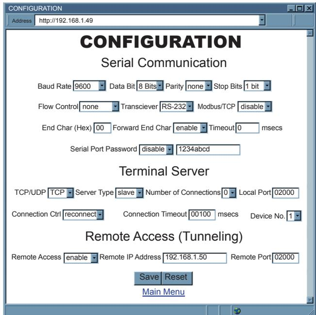
**Figure 4.16 Local iServer (Serial-to-Ethernet model) Configuration Page**
