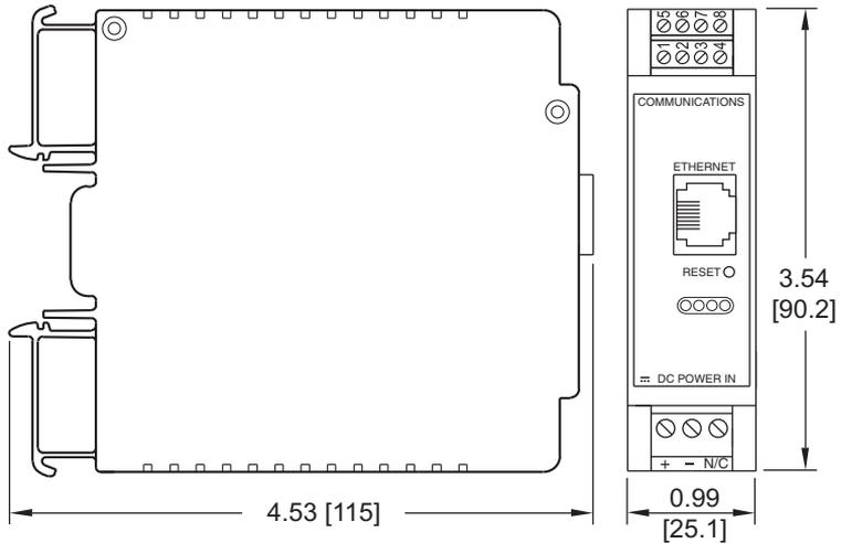
**Figure 5.2 DIN Rail iServer Dimensions**
