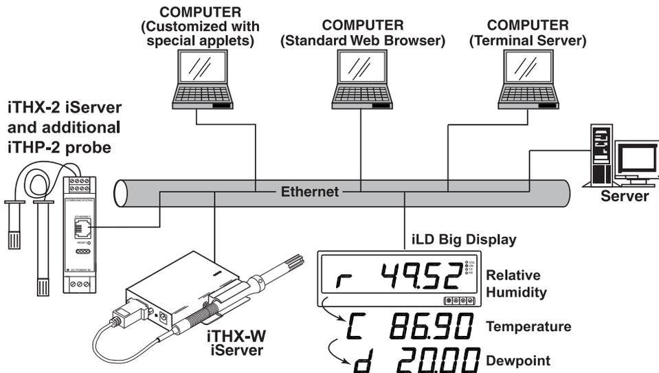
**Figure 1.1 iServer with Probe on the Ethernet Network**
