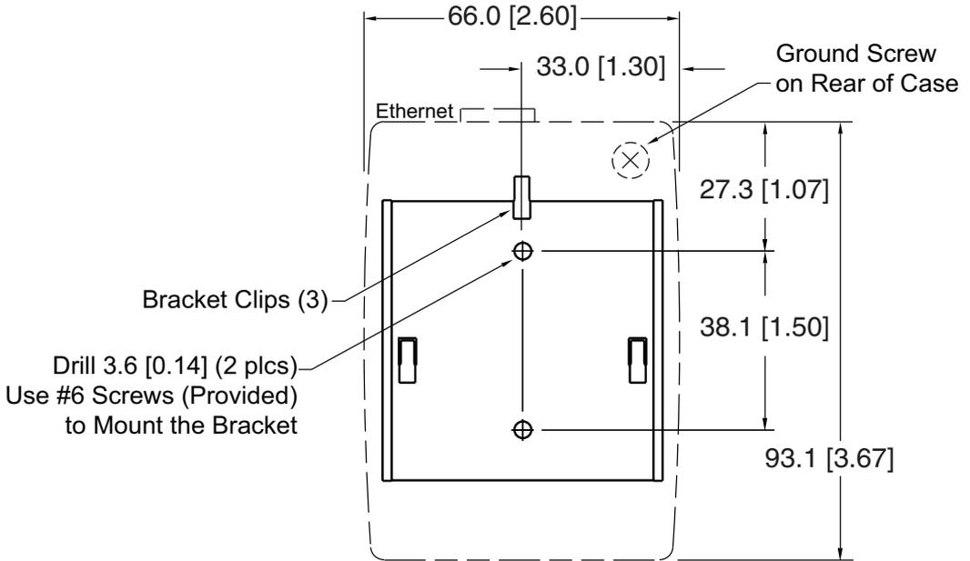
Figure 2.1 Mounting - Wall Mount iServer
