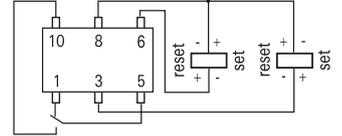
Contacts are shown in reset condition. Both coils can be used either as set or reset coil. Contact position might change during transportation and must be reset before use.
