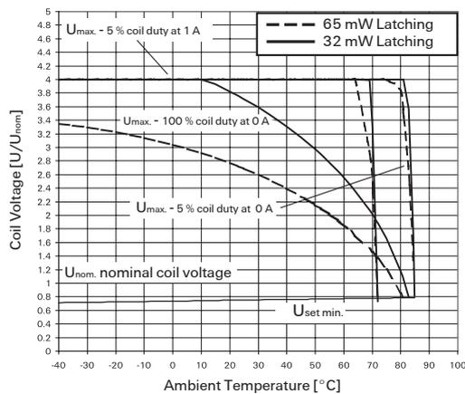
$U_{max}$  upper limit of the operative range of the coil voltage (limiting voltage) when coils are continuously energized.
