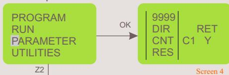
When the cursor is on PARAMETERS option and OK is pressed then screen 4 will be displayed.
