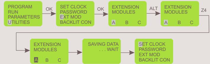
If only one extension module is being used and it has been assigned as 'A' on the extension module using the selection switch then make sure that 'A' is selected in the 'EXT MOD' option in the 'UTILITIES' menu. If more than one extension modules are being used then make sure that the modules have been assigned and selected appropriately because this in turn will affect the inputs and the outputs.
