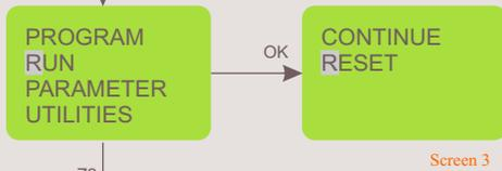
When screen 1 is being displayed, press the down key to shift the cursor to the RUN option and press OK key to enter it. Screen 3 will be displayed.
