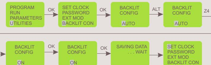
**AUTO:** In AUTO mode, whenever a key is pressed the backlit will be switched ON and will be switched OFF after 10 seconds.
