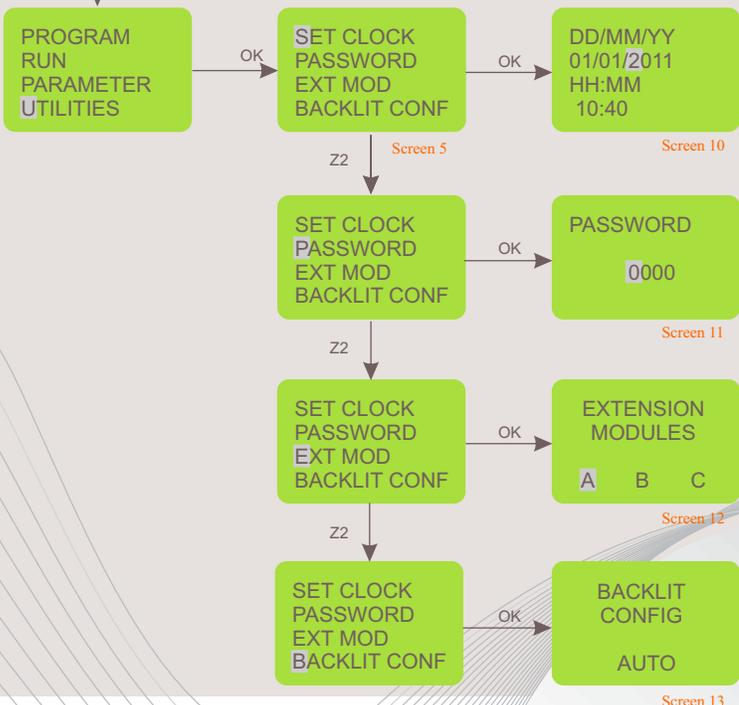
When the cursor is on the UTILITIES option and OK key is pressed, then screen 5 is displayed.
