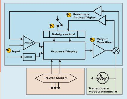
For industrial electronics, four channels allow you to perform three-dimensional testing, measuring input, output and feedback signals simultaneously.
