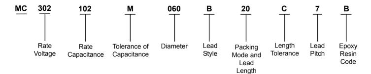
Rated Voltage: 302 = 3 KV dcRate Capacitance: 102 = 100 pFTolerance of Capacitance:  $M = \pm 20\%$
