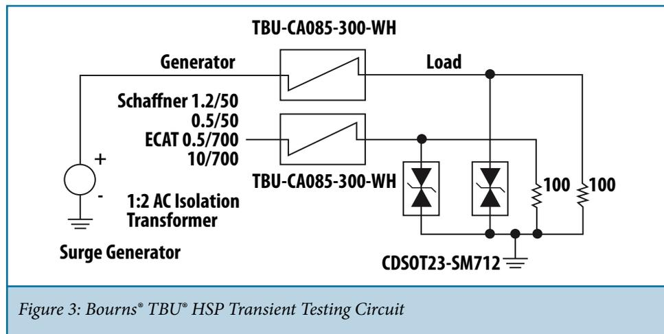
Figure 3: Bourns® TBU® HSP Transient Testing Circuit
