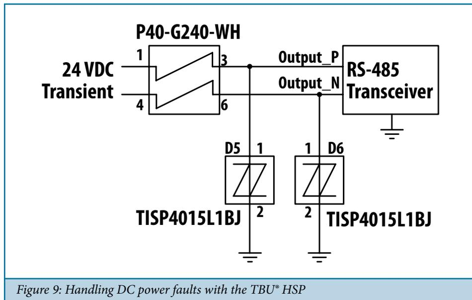
Figure 9: Handling DC power faults with the TBU® HSP
