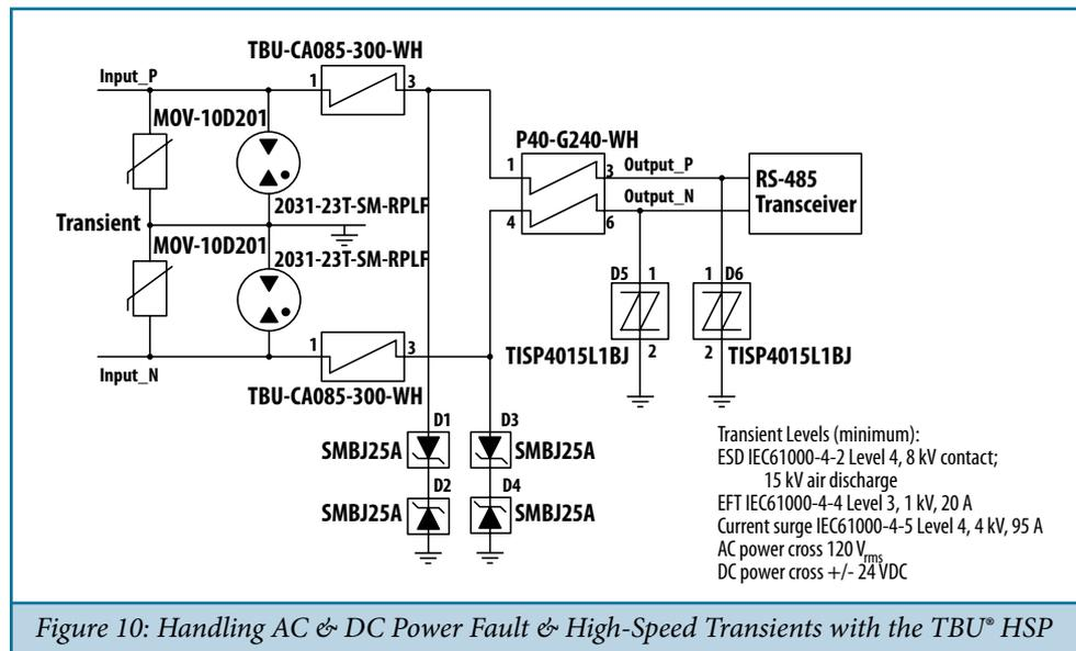
Figure 10: Handling AC & DC Power Fault & High-Speed Transients with the TBU® HSP
