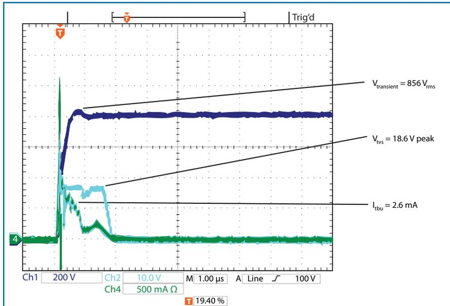
Figure 8: 0.5  $\mu$ s  $t_{rise}$ /700  $\mu$ s  $t_{fall}$  Surge
