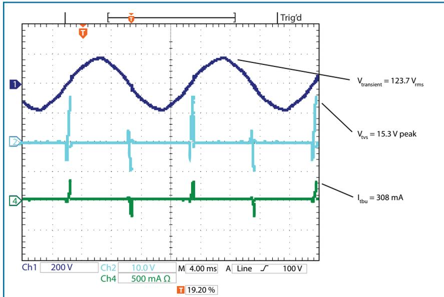
Figure 5: 120  $V_{rms}$  Power Cross
