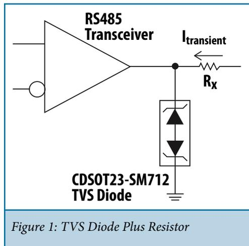
Figure 1: TVS Diode Plus Resistor
