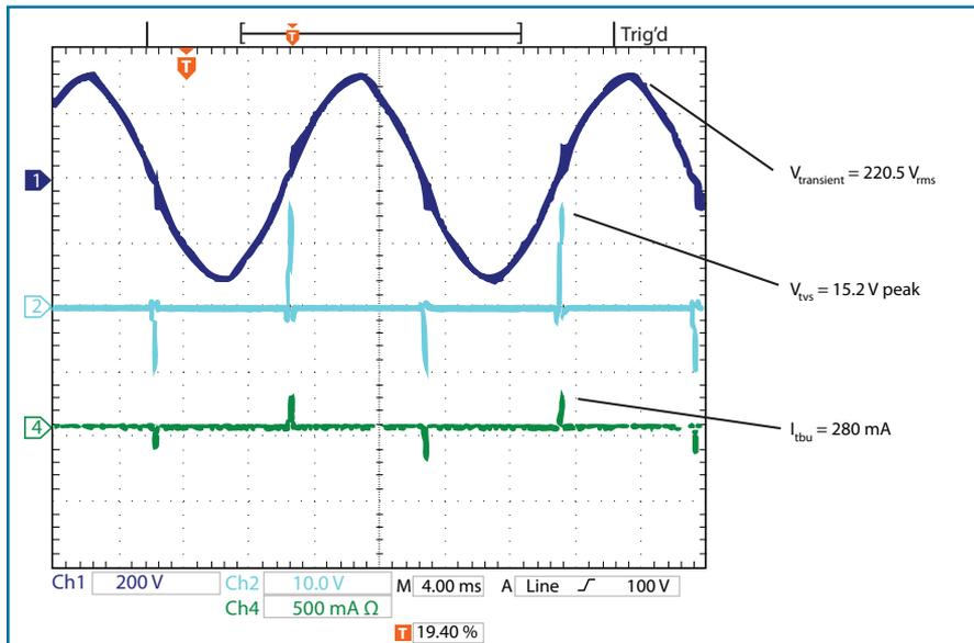
Figure 6: 220  $V_{rms}$  Power Cross
