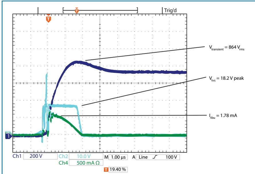
Figure 7: 1.2  $\mu$ s  $t_{rise}$ /50  $\mu$ s  $t_{fall}$  Surge
