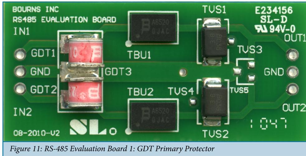
Figure 11: RS-485 Evaluation Board 1: GDT Primary Protector
