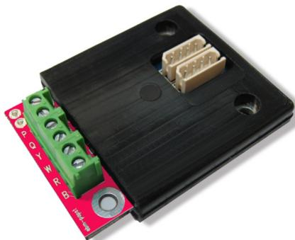
The A2P interface is a 0-10 volt to PWM converter and is designed to work with ebm-papst 4 wire PWM controlled DC fans. The interface translates the analogue voltage input to an equivalent PWM signal. The interface is matched to the fan so that with its very low power consumption, there is no need for a separate dedicated power supply.
