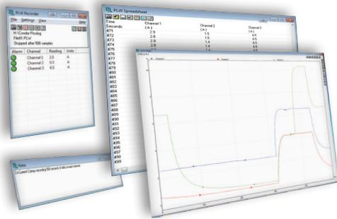
In addition to the monitor view, PicoLog can also display a graph, a spreadsheet and user notes. It can display them all at once, as shown here, or individually in any combination.
