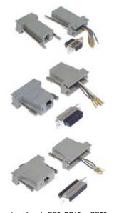
Adapts male or female DB9, DB15 or DB25 computer plugs to 8 position RJ45 or 6 position RJ11 modular socket. Back shell is pre-wired to modular socket ready to insert pins into desired positions of the DB connector.
