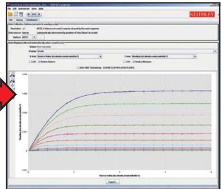
Performing nested sweeps to characterize a transistor with TSP Express is quick and easy. Data can be exported to a .csv file for use with spreadsheet applications such as Excel.
