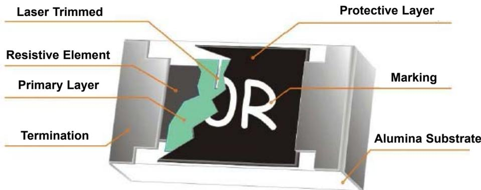
Figure 1. Construction of a Chip-R
