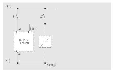
Control with parallel connected load
