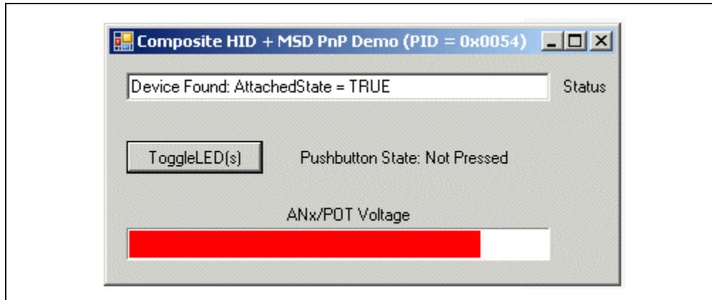
The demo PC application provides a simple graphical user interface for sending and receiving small amounts of example data to and from the HID interface on the USB device. Full source code for both this PC application and the demo firmware are included in the MCHPFSUSB Framework. Assuming the MCHPFSUSB Framework has been installed in the default location, the source code for both the firmware and PC application are found in the following directory:
