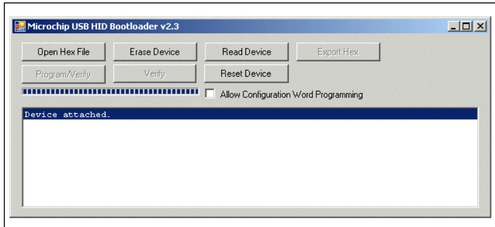
Once the PC application has found the USB device, the application can be used to open the Intel® HEX 32-bit formatted \*.hex firmware images and program them using the respective buttons.
