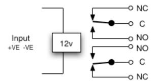
This relay is polarised and is therefore suitable for alarm bell circuits. It must be wired the correct way round for it to operate.
