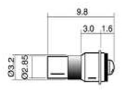
Dimensions in mm (typical) Not to scale Green dot on base of product signifies centre contact cathode -ve Colour sleeve on product denotes LED colour
