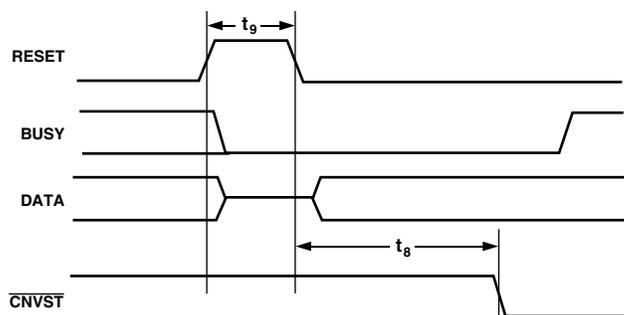
Figure 9. RESET Timing
