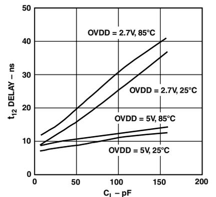
TPC 9. Typical Delay vs. Load Capacitance  $C_L$
