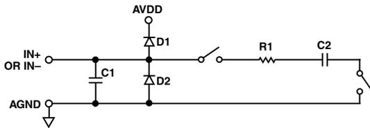
Figure 6. Equivalent Analog Input Circuit
