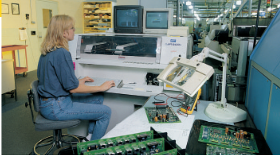
Automatic inline Takaya testing assures only good boards get to final assembly.
