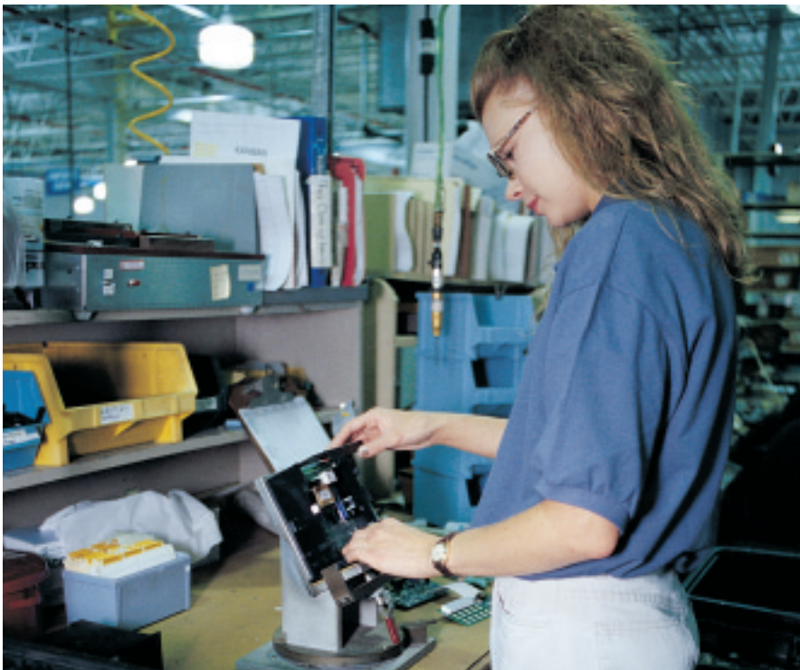
Component leads are formed prior to insertion into PCBs.
