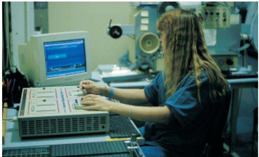
Microprocessors and memory are programmed for specific models.
