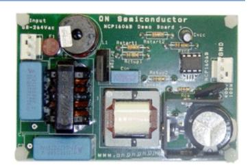
unity power factor across a wide range of input voltages and power levels. Housed in a DIP8 or SOIC -8 package, the NCP1606 minimizes the number of external components. Its integration of comprehensive safety protection features makes the NCP1606 an excellent driver for rugged PFC stages.
