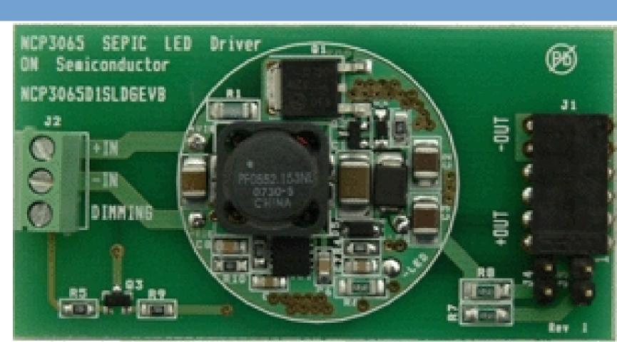
used to regulate the average current of the LED string. In addition, the NCP3065 has a wide input voltage up to 40 V to allow it to operate from 12 Vac or 12 Vdc supplies commonly used for lighting applications as well as unregulated supplies such as Lead Acid batteries.
