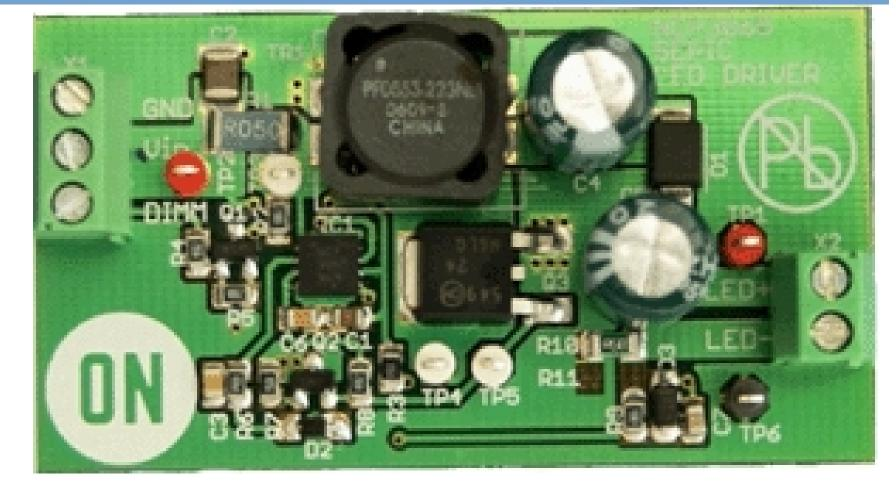
included. The circuit is based on NCP3065 operation at 250 kHz in a non -isolated configuration. The primary advantages of this circuit are in the wide input voltage range, wide output voltage range, and in its high efficiency. A pulse feedback resistor (R8) is used to vary the slope of the oscillator ramp, achieving duty cycle control and steady switching frequency over a wide input voltage range.
