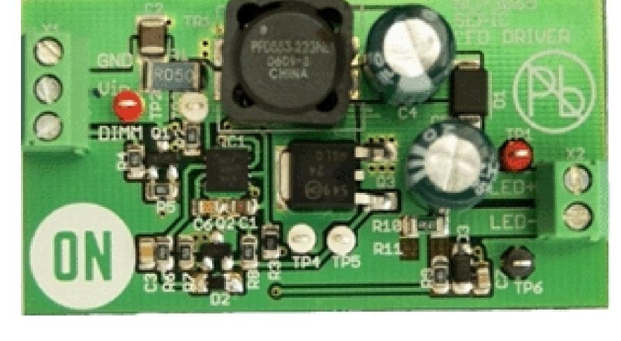
based on NCP3065 operation at 250 kHz in a non -isolated configuration. The primary advantages of this circuit are in the wide input voltage range, wide output voltage range, and in its high efficiency. A pulse feedback resistor (R8) is used to vary the slope of the oscillator ramp, achieving duty cycle control and steady switching frequency over a wide input voltage range.
